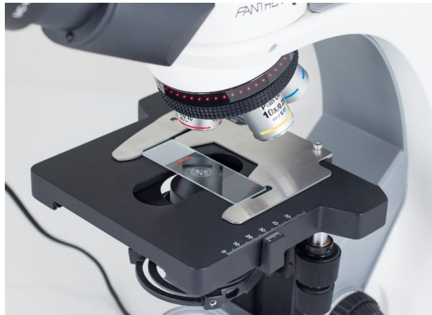
Figure 1: Stage, with slide properly positioned, of the Compound Light Microscope (Motic Panthera E2)
